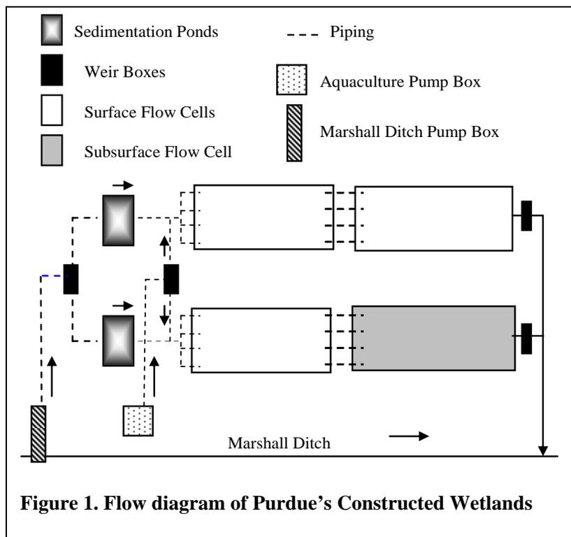
**Figure 1. Flow diagram of Purdue’s Constructed Wetlands**
