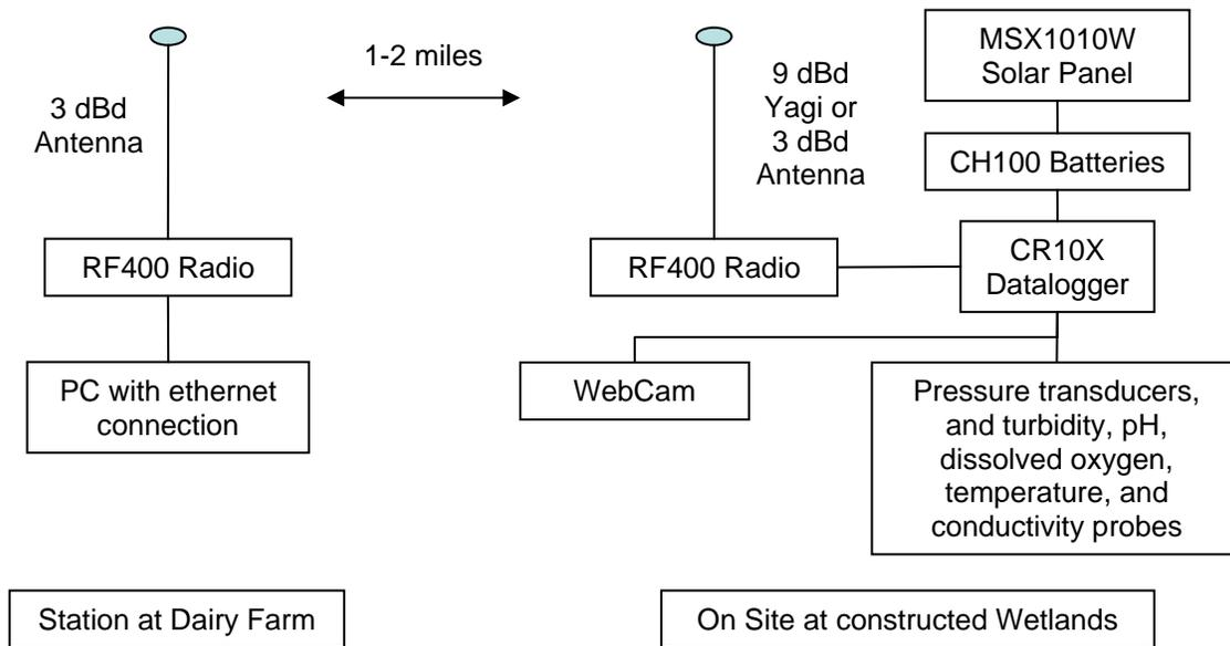
**Figure 2. Schematic of the proposed wireless monitoring system**
