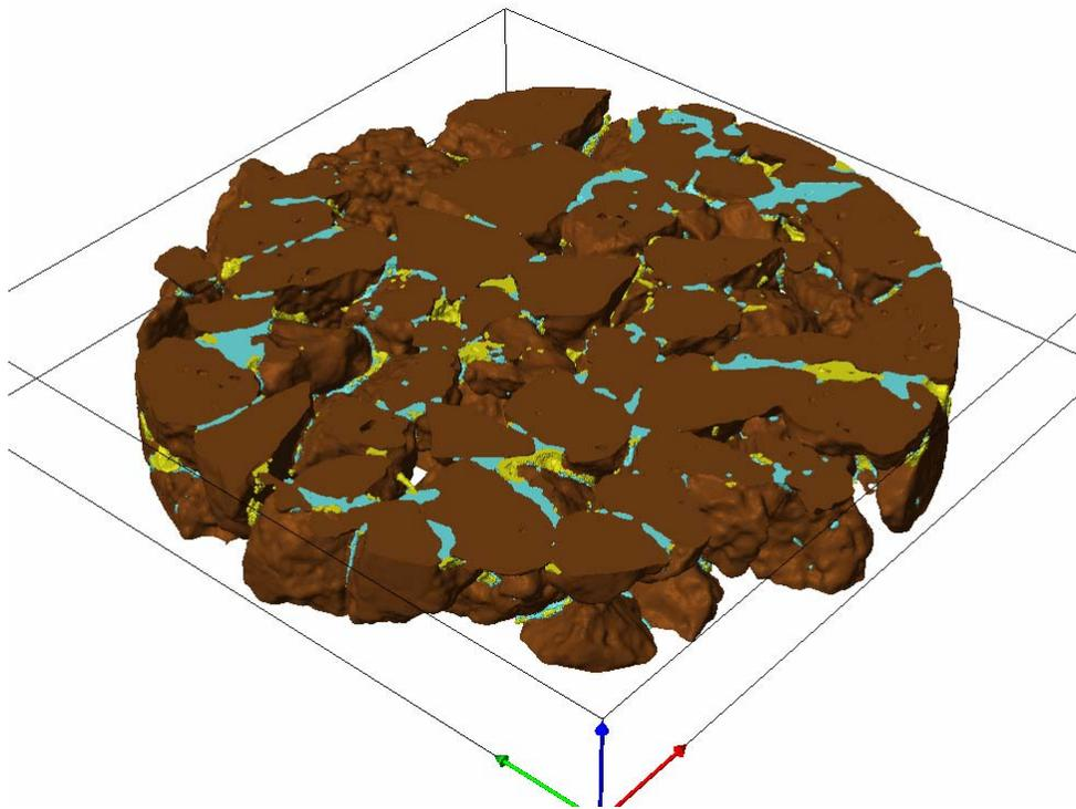
**Figure 3: Three dimensional reconstruction of zeolite infiltrated with a NaI solution and gasoline. The NaI solution is blue in color and the gasoline is gold.**
