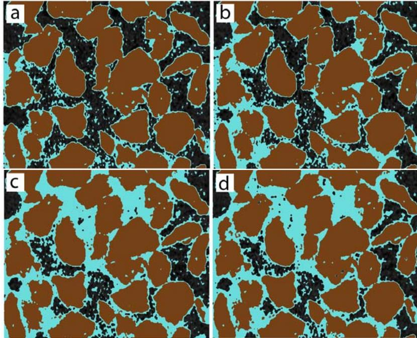
**Figure 1: Four vertical cross-sections representing the infiltration of water into the zeolite. The brown is the zeolite and the blue is the ice.**
