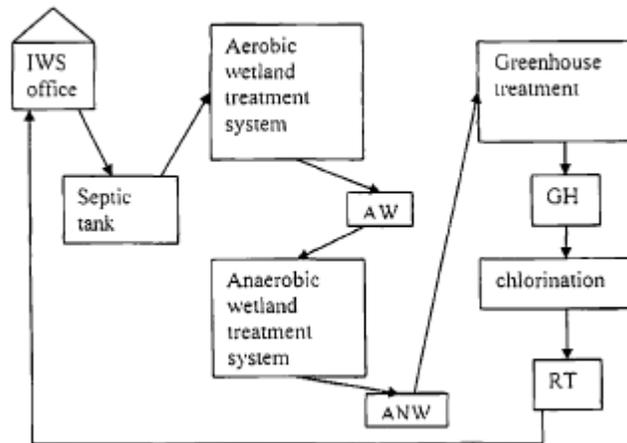
Figure 1. Integrated Water Systems Office (Chatham County) Septic System Design (AW, ANW, GH, RT are the sampling locations)
