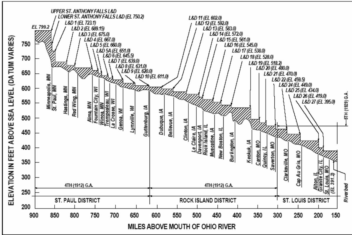
Figure 2. Schematic View of the Upper Mississippi River Pool System
