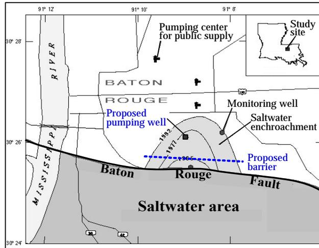
**Figure 1. The study site: saltwater encroachment toward pumping centers in the 1,500-foot sand aquifer, the proposed saltwater intrusion barrier, and the pump-and-treat remediation design (Modified from USGS website: [water.usgs.gov/wid/html/la.html](http://water.usgs.gov/wid/html/la.html))**
