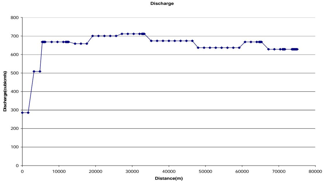
Figure 3: Steady flow discharges with the various inflows and outflows
