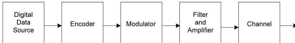
Figure 1: Schematic Diagram of the Transmitter for a digital Communication System
