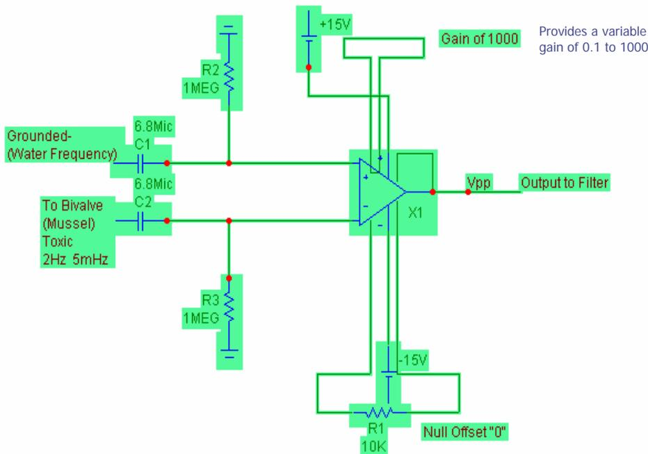
Figure 2: The preamplifier
