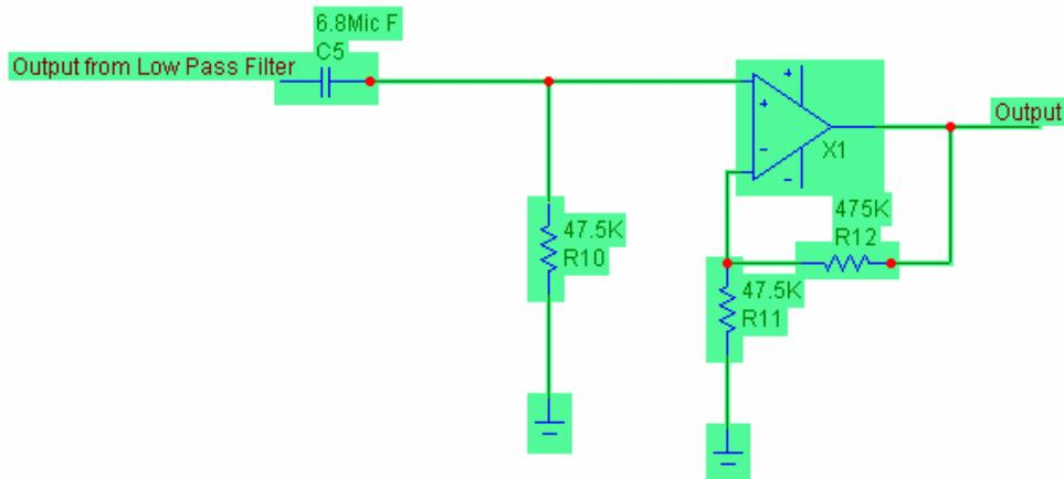
Figure 4: A high-pass filter design
