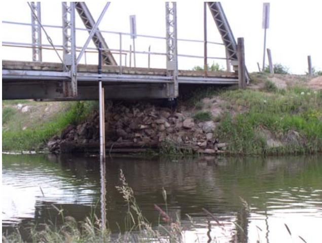
Figure 1 – Newly installed gaging station on the Bear River
