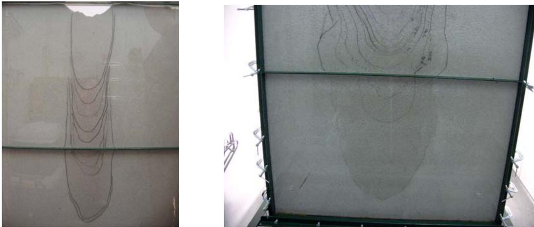
Figure 2. Plume shapes after approximately 18.5 hours for two flumes. The flume on the right has twice the water content prior to freezing as the plume on the left.
