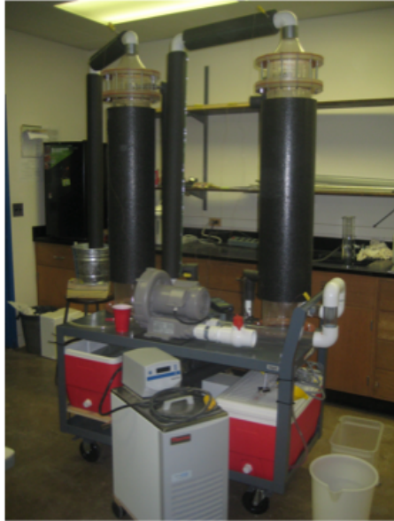
Figure 2. Picture of HDH desalination lab-scale experimental system.
