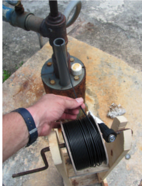
Figure 7: unwinding probe cable
