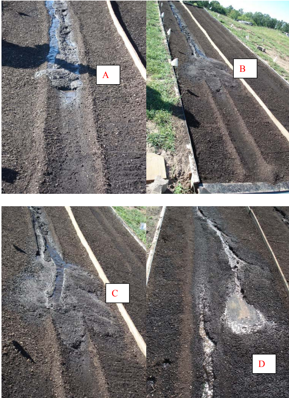
Figure 6. Pictures showing the micro-dams A: formed across the pre-created channel; B: grew as solids accumulate behind it; C: blew out allowing flow to advance; D: New micro-dam was formed encouraging more infiltration.
