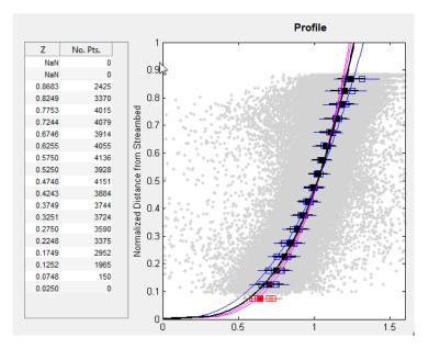
segment. The location of the mean normalized depth for each segment and number of points used in each segment is reported in a table to the left of the graph. The median value was selected to minimize the effect of any outliers.
