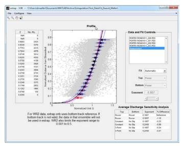
The theoretical logarithmic velocity profile is based on normalize depths with zero being at the streambed. When an average is computed with variable depths in WinRiver II depth cells at different normalized depths are averaged together, which is incorrect. To avoid this problem extrap computes the relative depth of each depth cell and then groups the depth cells into 5% increments of normalized depth to provide a representation of the average profile.
