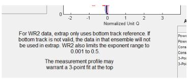
evaluation may be displayed. Although the 3-point top extrapolation method is included in the sensitivity analysis it is not included as a top extrapolation option in the Data and Fit Controls and will not be selected when using automatic fit algorithms. If the data meet criteria that suggest a 3-point top extrapolation may be appropriate, a message will appear in this area. A statement on the limitations of extrap for TRDI data is also displayed when appropriate.
