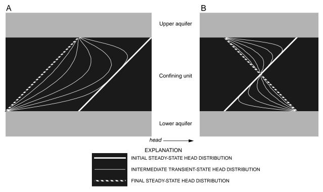
**Figure 2.** Distributions of head in a confining unit before and after head changes in overlying and underlying aquifers. Assumed initial conditions are steady-state flow from upper to lower aquifer. *A*, Head decreases equally in upper and lower aquifers. *B*, Head decreases in upper aquifer and increases in lower aquifer. Adapted from Trescott and others (1976).
