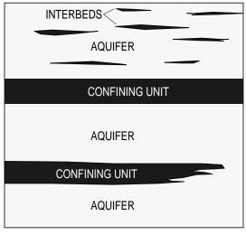
**Figure 1.** Types of fine-grained strata in aquifer systems. Confining units are laterally extensive and can divide coarse-grained material into individual aquifers. Fine-grained interbeds are laterally discontinuous beds within an aquifer.
