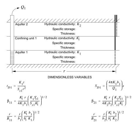
**Figure 8.** Conceptual model and dimensionless variables for analytical solution for drawdown in a two-aquifer system (Neuman and Witherspoon, 1969).
