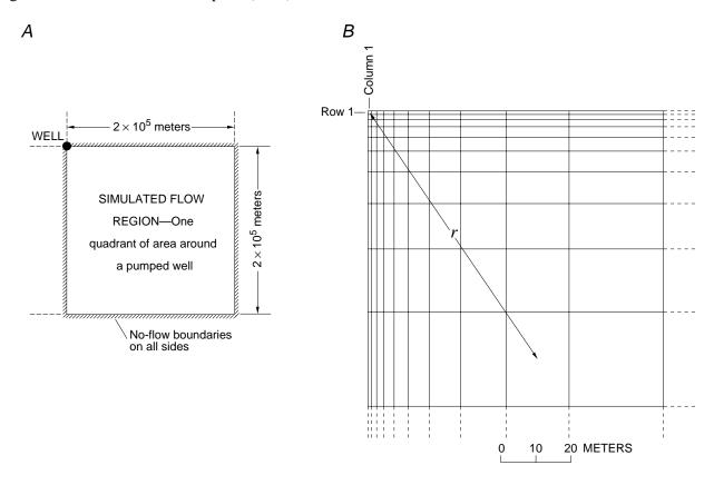
**Figure 9.** Modeled area for problem 2. *A*, Dimensions and boundary conditions for quadrant of area around pumped well. *B*, Part of model grid near pumped well.
