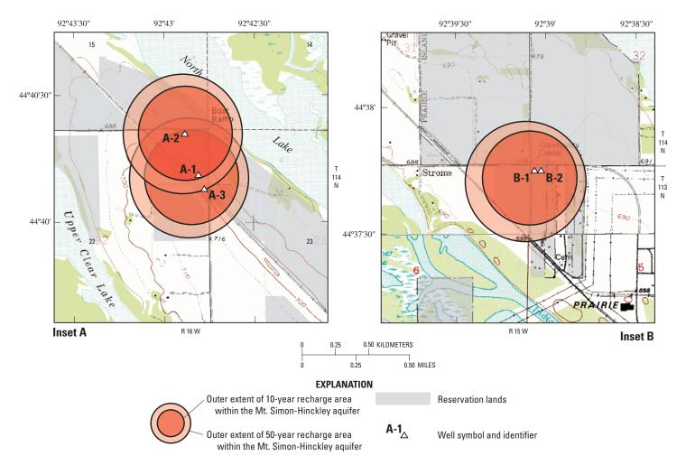
Figure 3. Recharge areas within the Mt. Simon-Hinckley aquifer to well fields A and B based on a rate of withdrawal of 625 cubic meters per day for each well field, Prairie Island Indian Community, east-central Minnesota.
