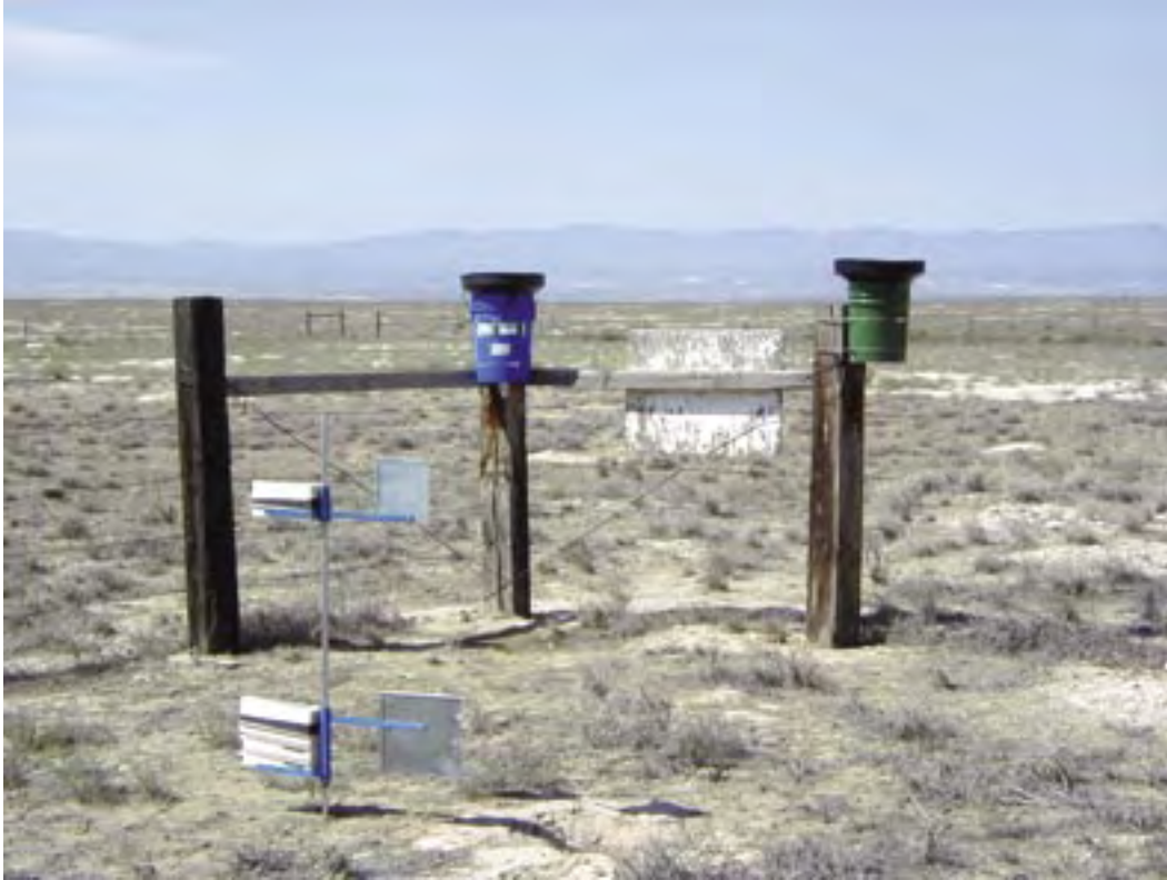
Figure 7a. Precipitation, airborne dust, and BSNE collectors, Orchard Training Area, Ada County, Idaho, Range 26 weather site, June 2002 (samples 62p and 62d)
