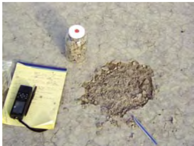
Figure 5. Sampling equipment and grab sample of soil at Tadpole Lake, Orchard Training Area, Ada County, Idaho, December 2002 (sample 50)
