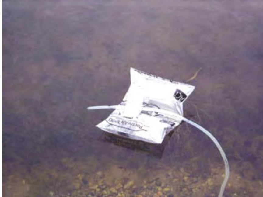
Figure 6f. MATES wash water pond, Orchard Training Area, Ada County, Idaho, March 2003, air-pillow support for sample tubing (sample17sw)
