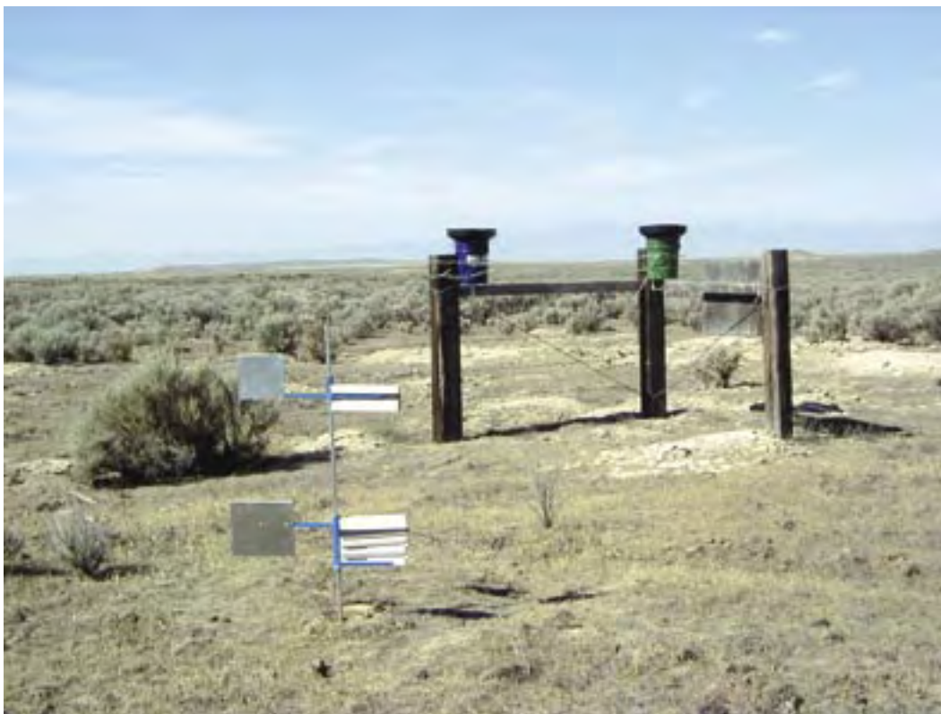
Figure 7b. Precipitation, airborne dust, and BSNE collectors, Orchard Training Area, Ada County, Idaho, Range 2 weather site, June 2002 (samples 30p and 30d)
