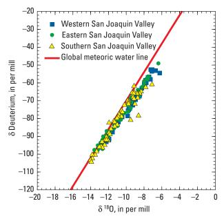
**Figure 26.** Stable isotopes  $\delta$  deuterium (<sup>2</sup>H) versus  $\delta^{18}$ O of ground water in the San Joaquin Valley, California, United States. H, hydrogen; O, oxygen;  $\delta$ , delta. Position of the global meteoric water line from Drever (1982).
