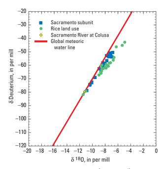
**Figure 27.** Stable isotopes  $\delta$  deuterium (<sup>2</sup>H) versus  $\delta^{18}$ O of ground water in the Sacramento Valley and of the Sacramento River at Colusa, California, United States. H, hydrogen; O, oxygen;  $\delta$ , delta. Position of the global meteoric water line from Drever (1982).
