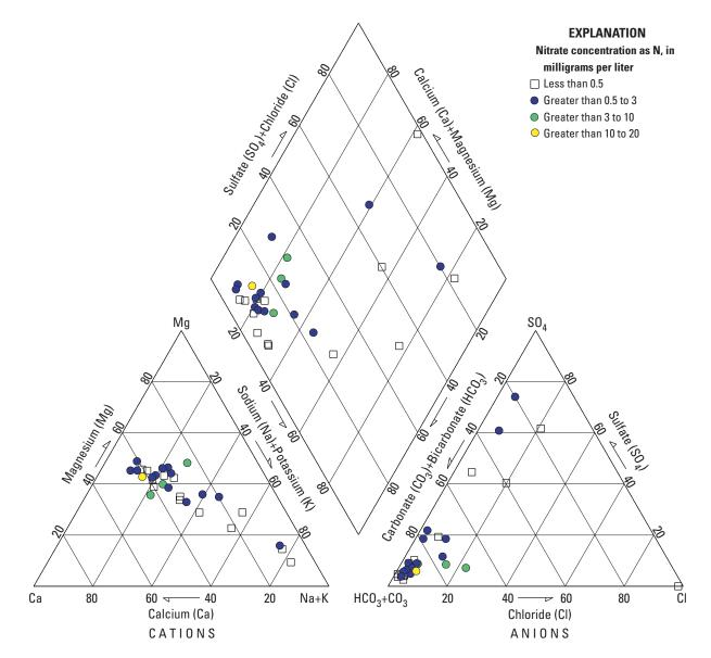
Figure 20. Trilinear graph of the rice land-use ground water, Sacramento, California, United States. Note: Red circles are not shown here because ground water with nitrate greater than 20 milligrams per liter was not detected. Each scale represents percentage of total milliequivalents per liter. N, nitrogen.
