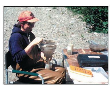
Figure 5. Hydrologist Tim Brabets sieving fine-grained streambed sediments Photograph by Steve Frenzel, 1998.
