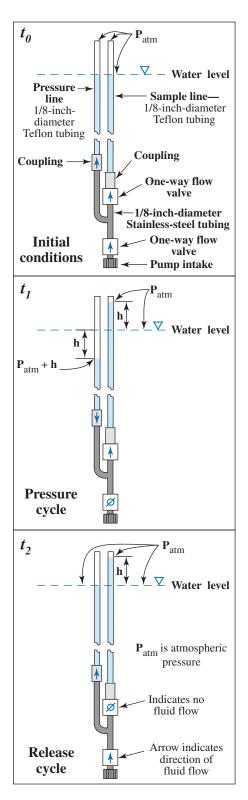
**Figure 1.** Diagram showing schematic of smalldiameter pump and basic operating principles. sample pump after pressure is released (Release cycle, fig. 1).
