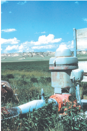
Irrigation well in Laramie County, Wyoming (Photograph courtesy of R.R. Luckey, U.S. Geological Survey.)
