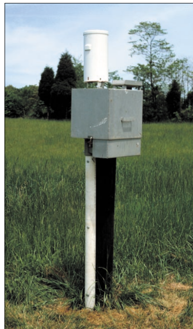
Well with tipping-bucket rain gage mounted on top.
