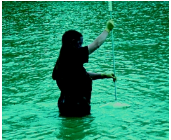
Figure 3. Equal-width increment sampling is done by wading where stream depths permit. (Photograph by C.A. Hartmann Jr., U.S. Geological Survey.)
