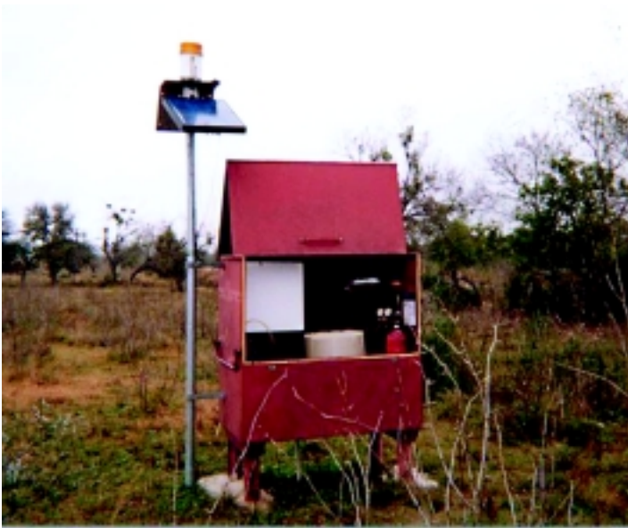
Figure 2. Typically, an autosampler (white object in center of shelter) is installed on relatively high ground with a sampling tube running underground to the stream. Power is supplied by batteries recharged by a solar panel (at left). (Photograph by C.L. Otero, U.S. Geological Survey.)
