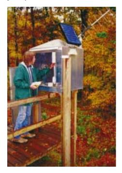
Figure 1. Satellite-linked stream gage on Crabtree Creek in Raleigh.
