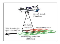
Figure 2. The scanning pattern of NASA's airborne topographic mapper.
