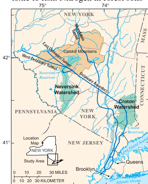
Figure 1. New York City water-supply system.
