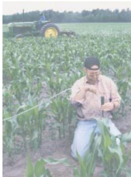
Figure 8. Sampling shallow ground-water for nutrients and pesticides.
