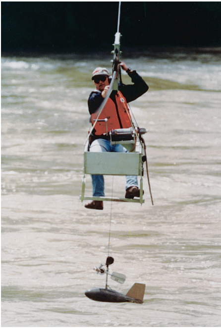
Figure 4. A USGS hydrologist collecting flood-flow data on the Snake River in eastern Idaho. (Photograph by Randy Hayes, Idaho Falls Post Register.)
