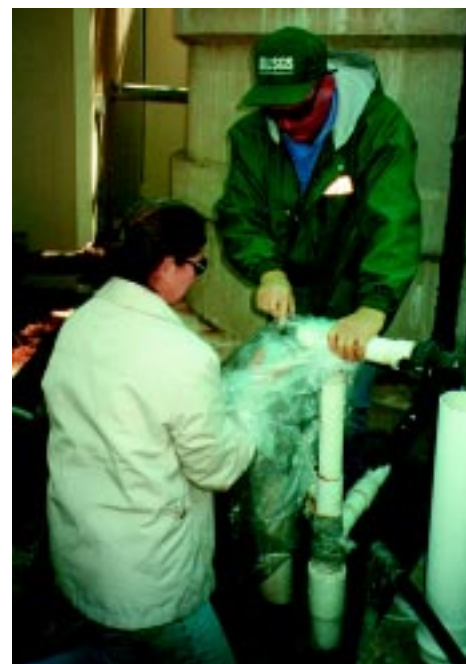
Personnel collecting a sample from a well. The sampling outlet is protected with a sheet of plastic to avoid contamination during sample collection.
