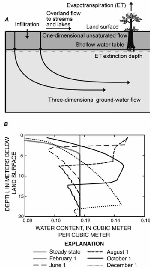
Figure 1. (A) 1D unsaturated zone flow simulated with the new UZF1 package for MODFLOW-2005 and (B) representative water-content profiles calculated by UZF1 for a model cell in a test simulation with time-varying infiltration rates at land surface. Figures modified from Niswonger et al. (2006b).
