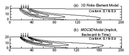
Figure 14. Three-dimensional simulation results for nonuniform-flow test case in which  $_{TH} = _{TV} = 0.1 \text{ m}$ : (a) finite-element model (modified from Burnett and Frind, 1987, figure 9b), and (b) implicit *MOC3D* solution using backward-in-time approximation and CELDIS = 0.5. Plume positions are represented by contours of relative concentration in vertical plane of three-dimensional grid; contour interval is 0.2 relative concentration.
