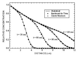
Figure 7. Numerical (implicit) and analytical solutions for four different times for solute transport in a one-dimensional, steady flow field for case with decay at rate of  $= 0.01 \text{ s}^{-1}$ .
