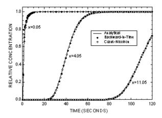
Figure 4. Numerical (implicit) and analytical solutions at three different locations for solute transport in a one-dimensional, steady flow field. Parameter values for this base case are listed in table 6.
