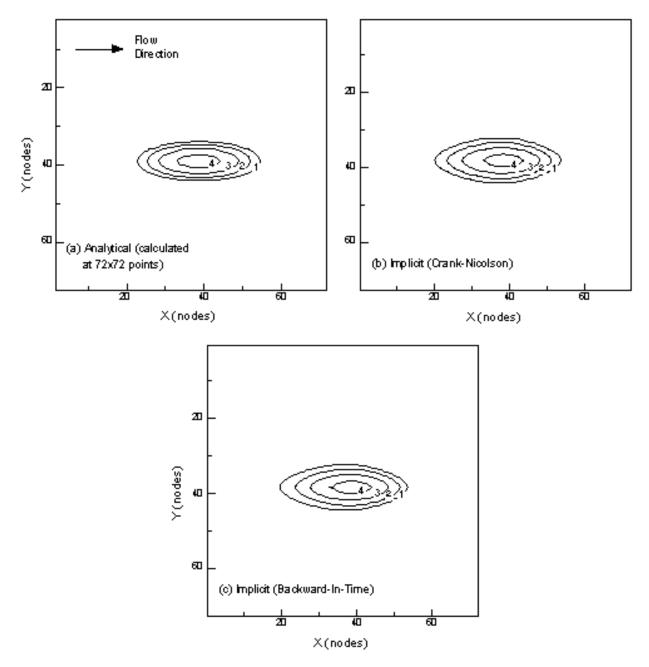
Figure 9. Concentration contours for (a) analytical and (b, c) numerical solutions for transport of a point initial condition in uniform flow in the *x*-direction. The *z*-component of flow is zero, but there is dispersion in all three directions. Contour values are the log of the concentrations.
