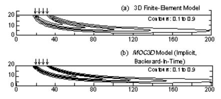
Figure 13. Three-dimensional simulation results for nonuniform-flow test case in which  $_{TH}$  = 0.1 m and  $_{TV}$  = 0.01 m: (a) finite-element model (modified from Burnett and Frind, 1987, figure 8c), and (b) implicit *MOC3D* solution using backward-in-time approximation and CELDIS = 0.5. Plume positions are represented by contours of relative concentration in vertical plane of three-dimensional grid; contour interval is 0.2 relative concentration.
