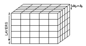
Figure 2. Representative three-dimensional grid for *MOC3D* illustrating notation for layers.
