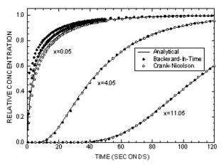
Figure 5. Numerical (implicit) and analytical solutions at three different locations for solute transport in a one-dimensional, steady flow field for case of increased dispersivity ( $_L = 1.0$  cm,  $D_{XX} = 0.1$  cm<sup>2</sup>/s, and other parameters as defined in table 6).
