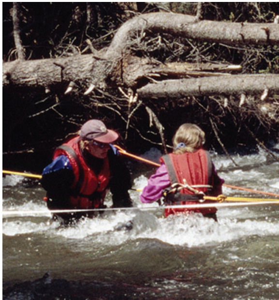
Figure 54 —Operating bedload traps in poorly wade-able flow. Hazardous downstream flow conditions warrant increased safety measures such as life vests, climbing harnesses, and ropes for each operator's belay. Crossing the ropes should be avoided and operators should be experienced in handling belays. Photo courtesy of Winema National Forest, Klamath Falls, OR.
