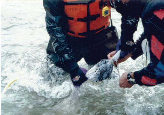
Figure 38 —Operator 1 holds the end of the net above and below the accumulated debris while operator 2 unties the net.
