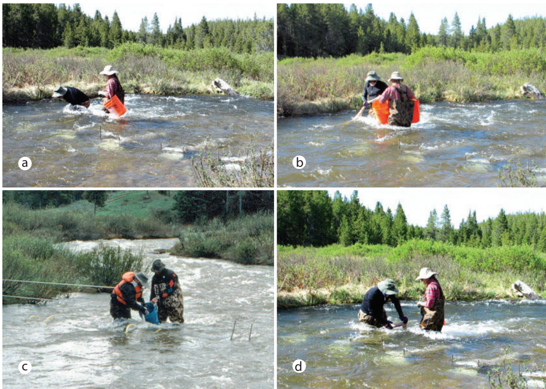
Figure 39 —Emptying bedload traps in the stream without a footbridge: grabbing the net (a), untying it (b), emptying the net into a bucket (c), and retying the net (d). Note: the persons in the right of each photo should be wearing wading belts!
