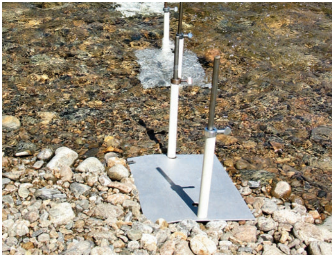
Figure 28 —Ground plates with PVC pipe pieces fastened with shaft collars.
