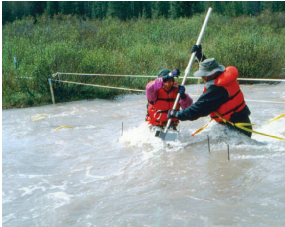
Figure 53 —Safety devices used by operators at high flow in Little Granite Creek. Notice the life vests and the safety rope fastened across the stream.
