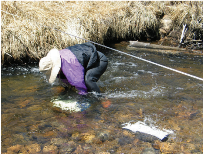
Figure 25 —Setting a ground plate onto the stream bottom.
