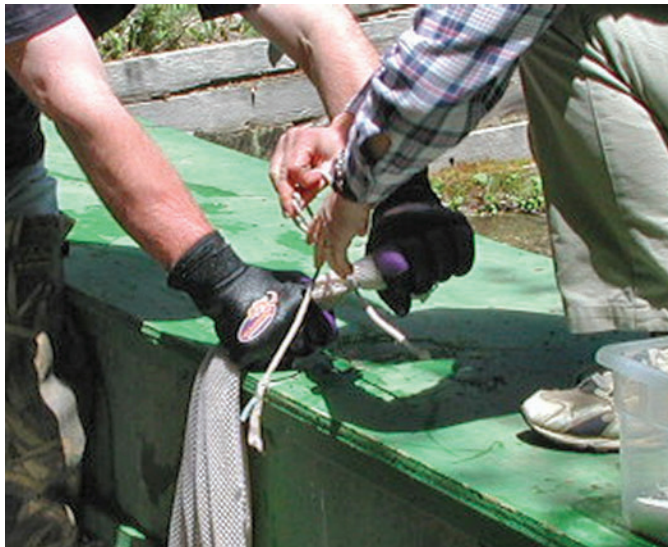
Figure 36 —Tying off a bedload trap at East St. Louis Creek (Photo courtesy of J. Potyondy, USFS Stream System Technology Center).
