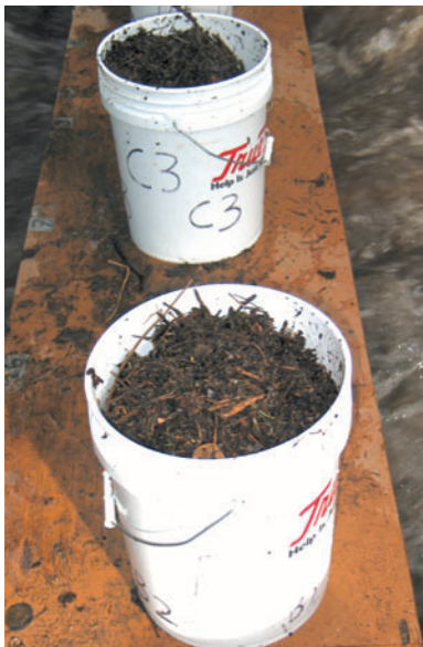
Figure 47 —4.5 gal of organic debris was collected in a 19-minute bedload trap sample.
