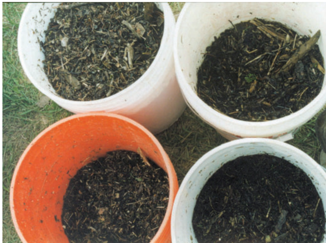
Figure 43 —Inappropriately large volumes of organic debris of up to 4 gal (approx. 16 liter) collected during a 1-hour sample in the bedload traps (upper left bucket).
