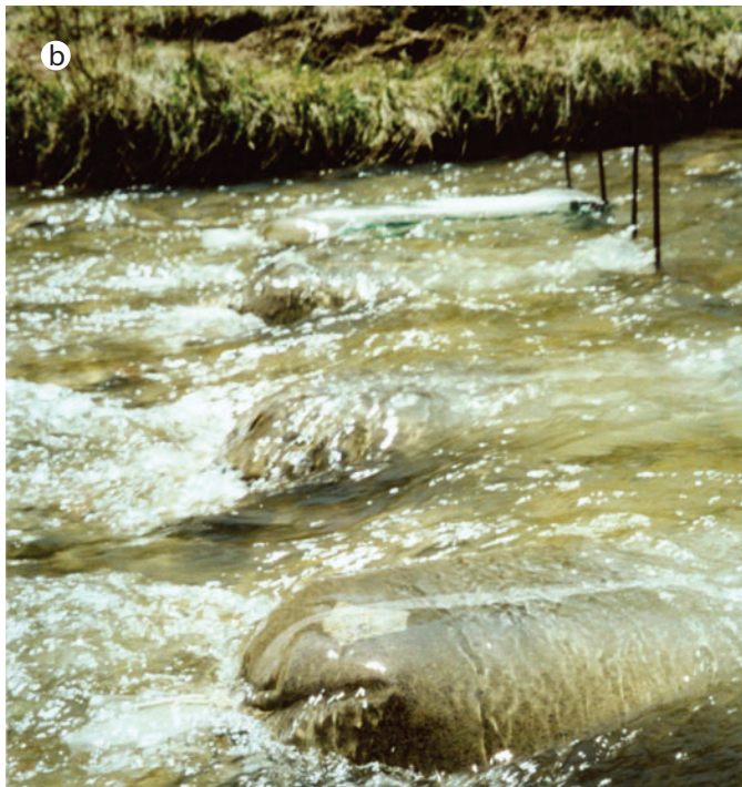
Figure 10 —Net with 0.5 mm mesh (a) bulging in the flow and severely ponding the water level upstream of the traps even at low flow (b).
