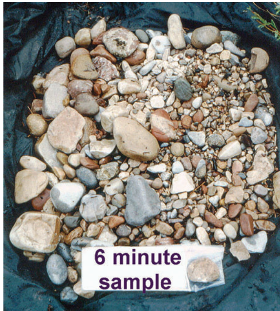
Figure 44 —Twenty kg of gravel and cobbles were collected in one of the bedload traps over a 6-minute sampling time when bedload sheets moved along the stream bed at Little Granite Creek, WY, in 1999.
