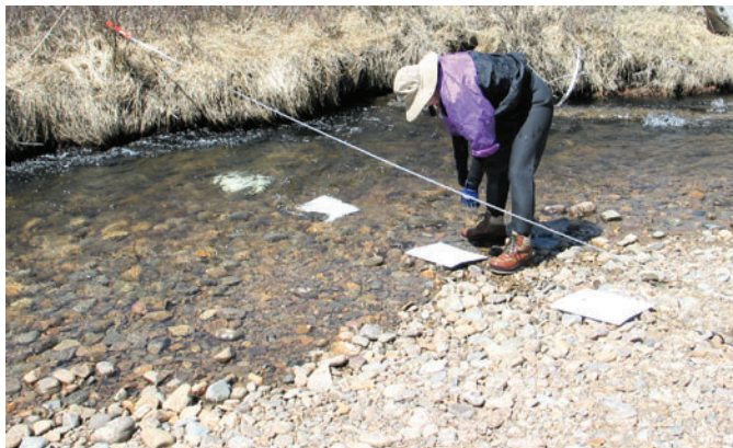
Figure 23 —Ground plates are laid out in a cross-section at low flow.
