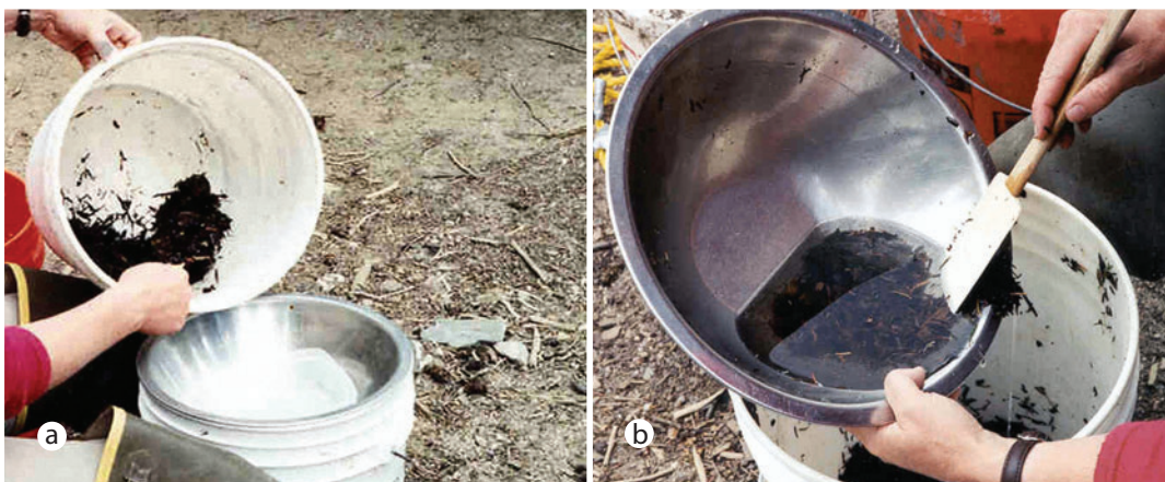
Figure 49 —The sample is poured into a metal bowl for washing (a). The sample is covered in water and stirred with a rubber spatula (b). Organic material is decanted and discarded.
