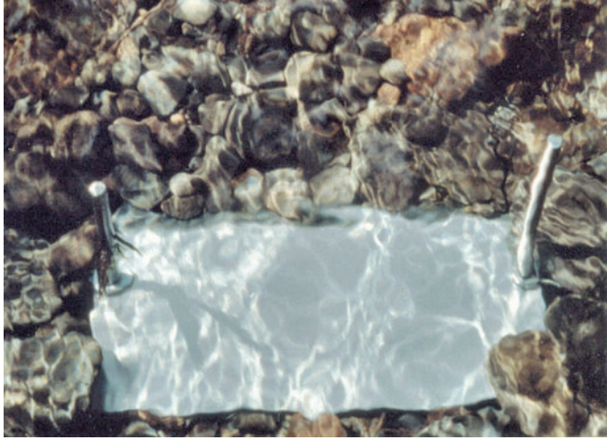
Figure 27 —Ground plates installed on the stream bed during low flow (view upstream).
