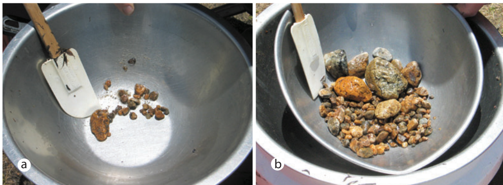
Figure 50 —Bedload particles are retained in the bowl, from a small sample (a) and a larger sample (b).
