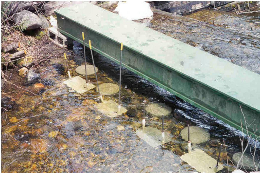
Figure 29 —Stepping stones placed behind ground plates in relatively fine gravel bed material at the East St. Louis Creek sampling site. Note the impractical, unnecessarily long stake lengths at the two ground plates near the left bank. The 16-ft long footbridge in the back is placed too close to the ground plates causing a cramped work space for the trap operator.
