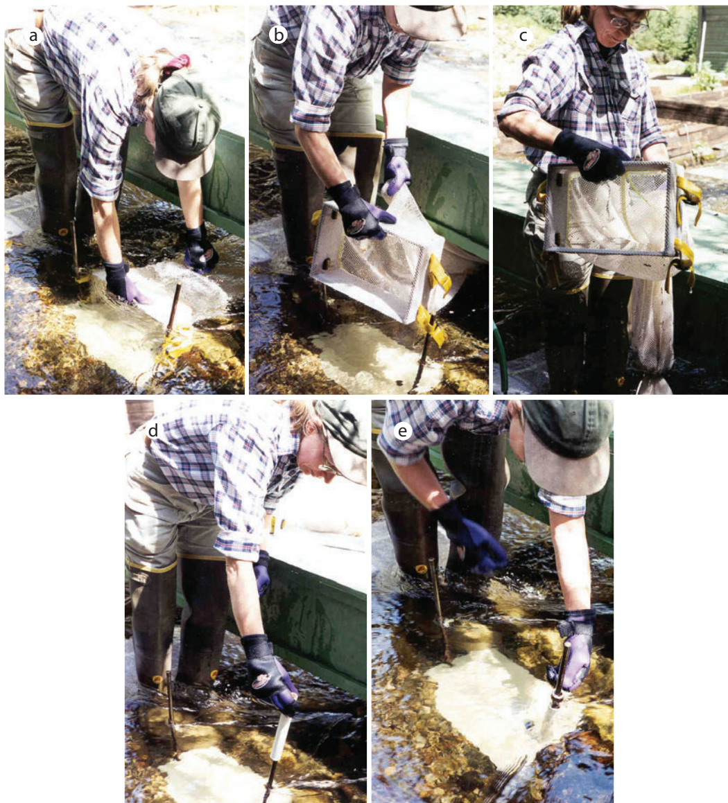
Figure 42 —Removing a bedload trap from its ground plate (see text for explanation).
