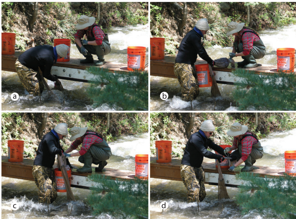
Figure 41 —Emptying bedload traps from a footbridge. Operator 1 grabs the net above the accumulated bedload (a) and lifts it out of the water and places the end of the net with the accumulated bedload onto the bridge (b). Crouching on the bridge, operator 2 unties the net and dumps the contents of the traps into a 5-gal bucket that operator 1 holds between himself and the bridge (c). Operator 2 places the sample bucket onto the bridge and reties the net (d).
