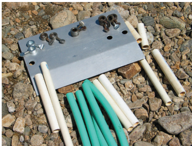
Figure 5 —Ground plate with inclined front edge, pieces of PVC pipe, and pieces of garden hose.
