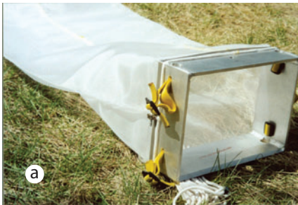
Figure 10 —Net with 0.5 mm mesh (a) bulging in the flow and severely ponding the water level upstream of the traps even at low flow (b).
