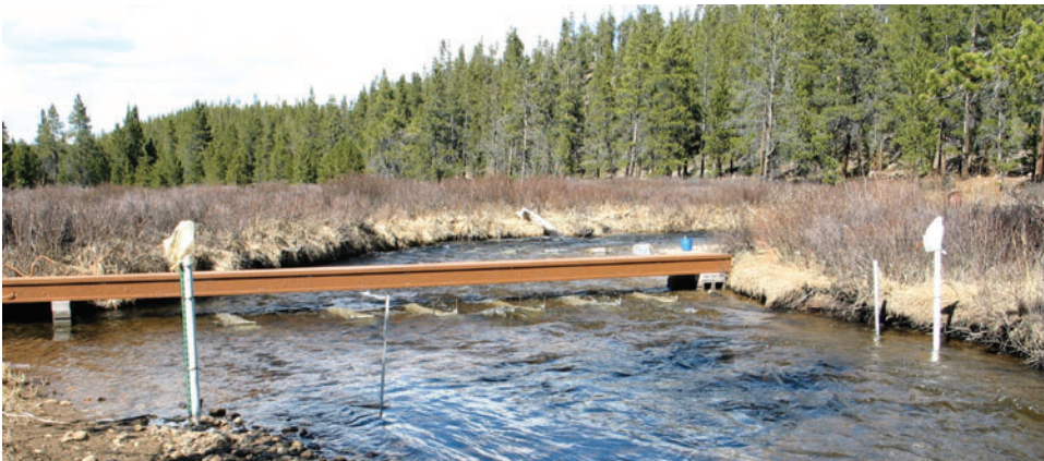
Figure 46 —Bedload trap sampling site with footbridge. Staff gauges and electronic water level recorders (inside the white PVC tubes) were installed upstream near both banks, conveniently close to the bridge, but were affected by the hydraulic resistance of the bedload traps.
