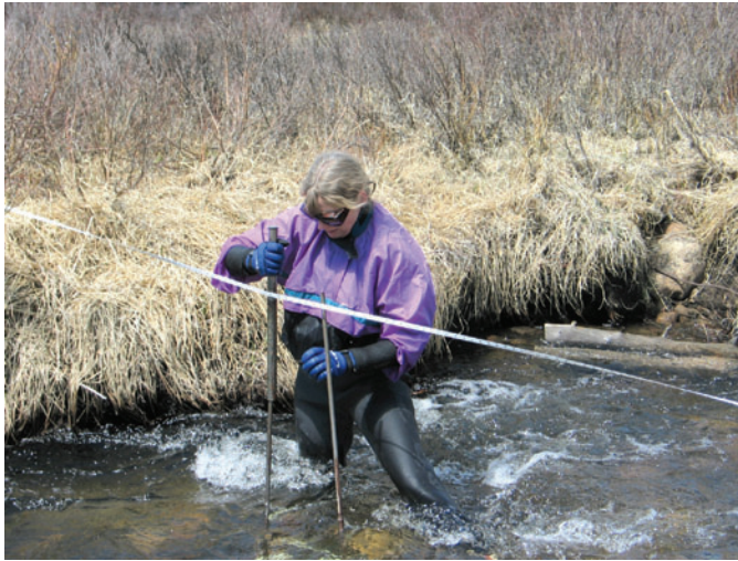
Figure 26 —Starting to drive the stakes in by sliding the stake driver up and down.
