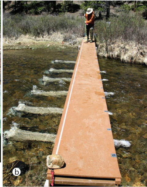
Figure 11 —3-ft long nets proved too short for emptying the net from a bridge. Note the cramped workspace for the operator in the stream (a) (Photo courtesy of J. Potyondy, USFS Stream System Technology Center); 5-to 6-ft long nets are more suitable (b).
