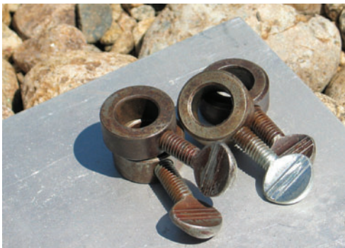
Figure 8 —Shaft collars with thumb screws to hold the webbing straps in place.
