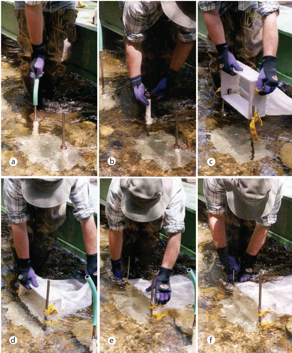
Figure 34 —Six steps of setting the bedload traps onto the ground plates: Removing the hose pieces (a), removing the shaft collar (b), sliding the webbing loops over the stake (c), pushing the trap down onto the ground plate (d), checking the trap position (e), and fastening the shaft collar (f).
