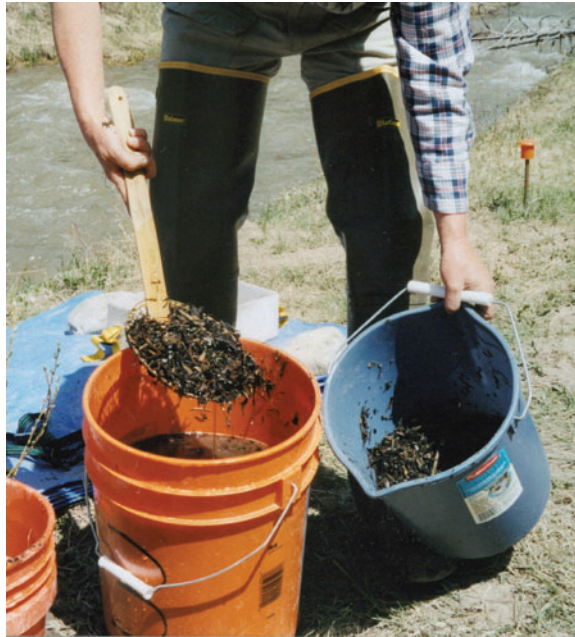
Figure 51 —Washing a sample with large amounts of organic material using a big wire spoon.
