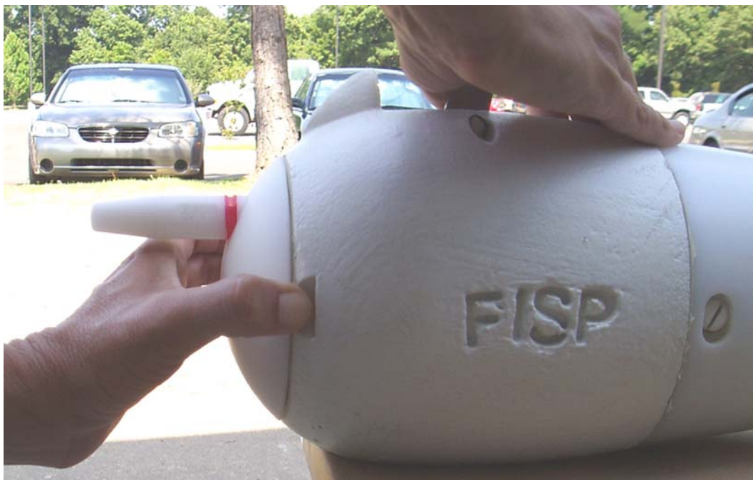
Figure 13-- To remove sample, grab nose-piece at sampler body indentions
