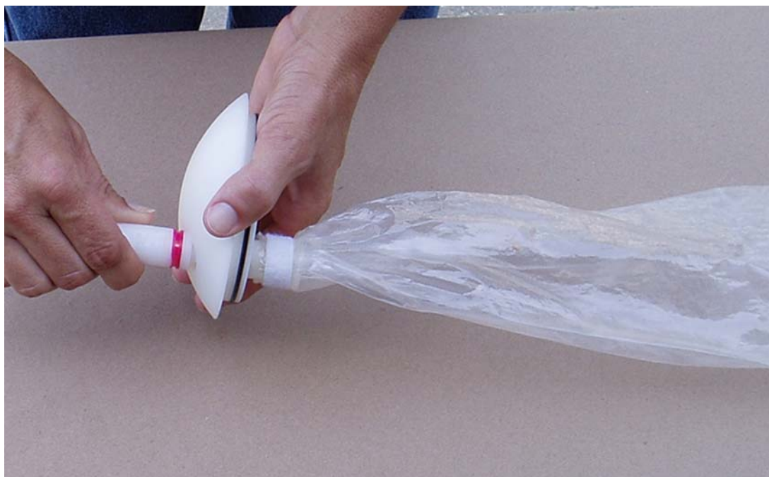
Figure 6-- Screw nozzle into nozzle holder
