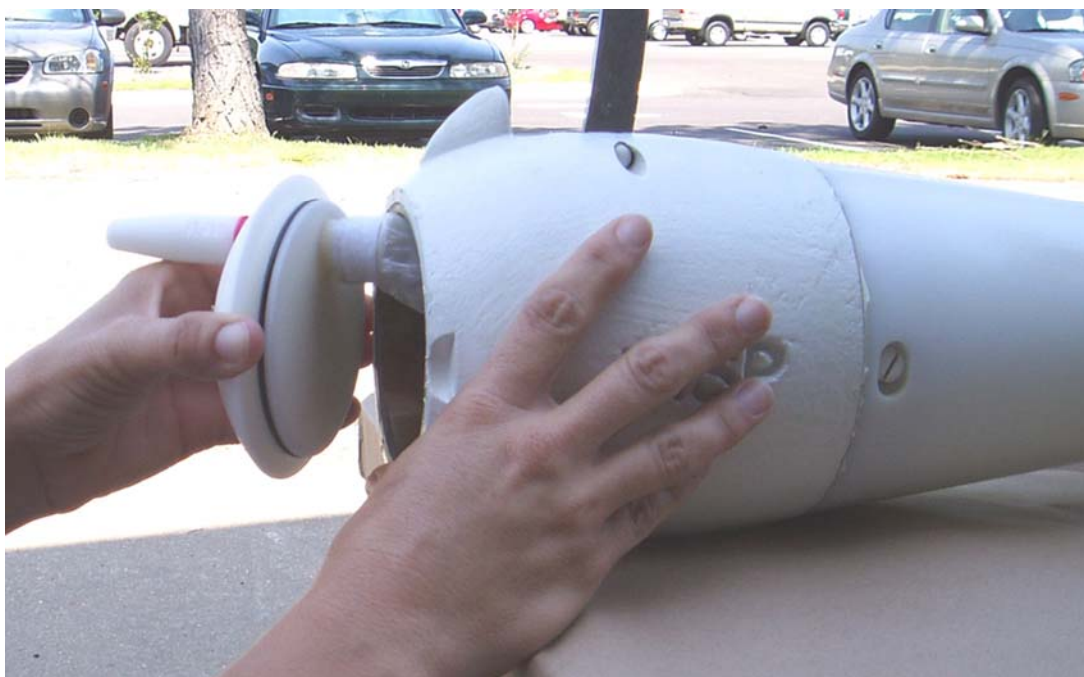
Figure 14-- Pop the nose-piece from sampler body and remove sample
