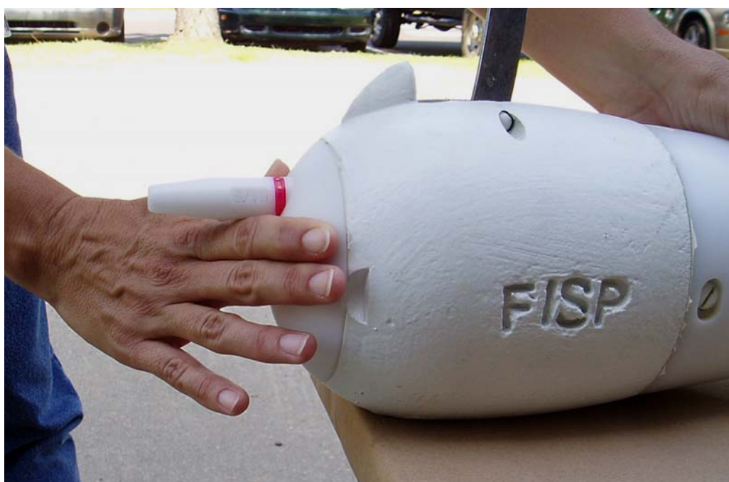
Figure 12-- Snap the nose-piece into the sampler cavity
