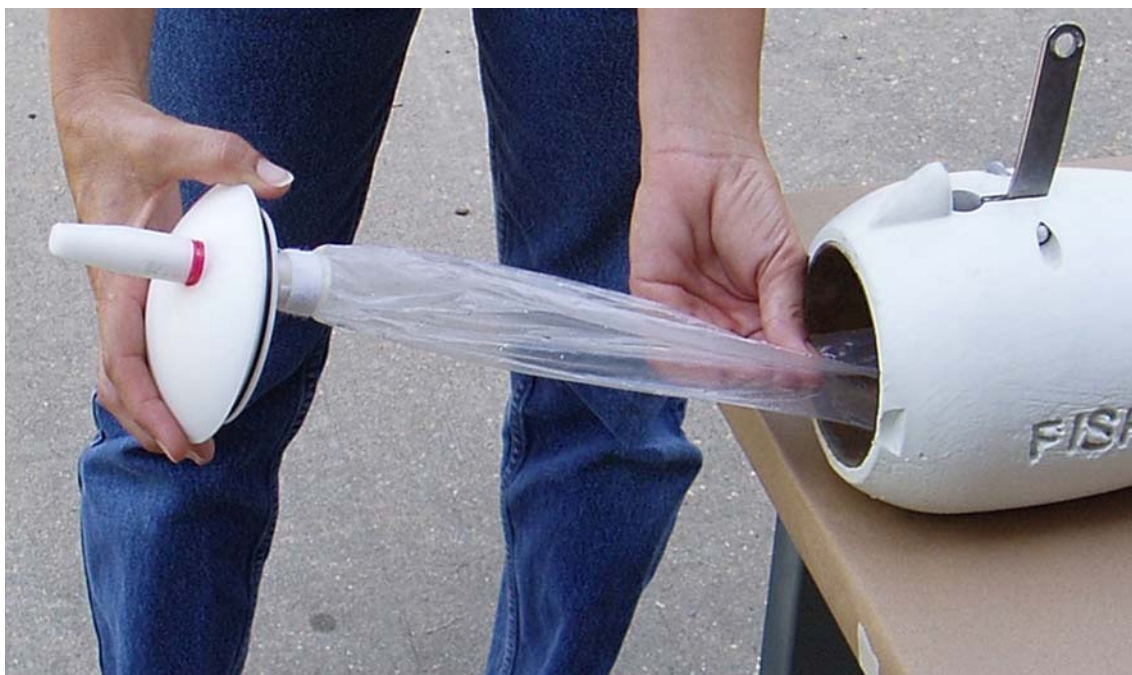
Figure 9-- Push the air out of the folded bag
