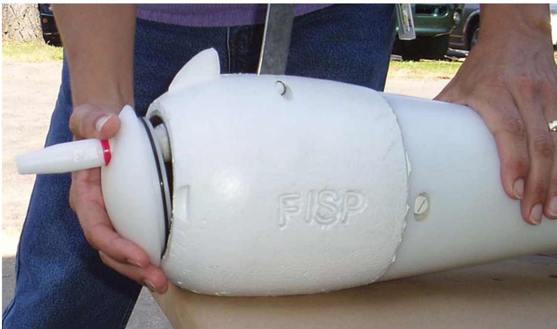
Figure 11-- Insert the bottom of the nose-piece into bottom of sampler cavity
