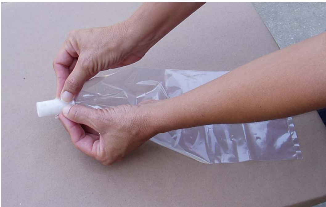
Figure 3-- “Gather” the bag opening around the nozzle holder
